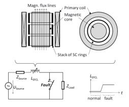
Figure 1: Schematic drawing of the shielding-core type inductive superconducting fault current limiter (top) along with the electric circuit in which it is embedded (lower left) and a graph showing the idealized change of the primary inductance (lower right)
